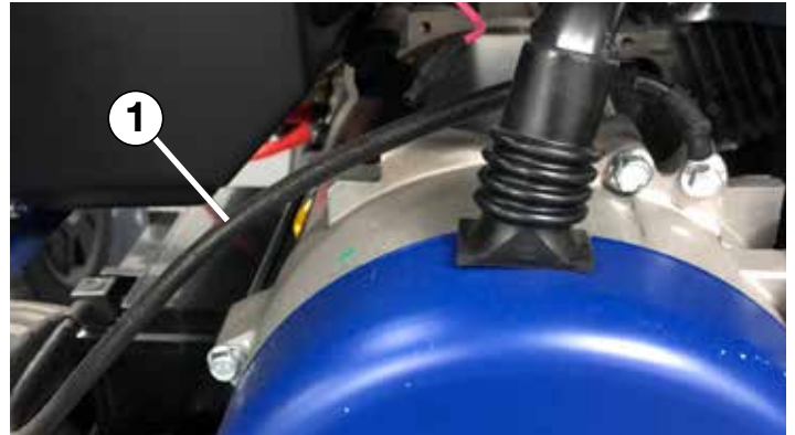
Figure 5 - Locating Negative (-) Cable
